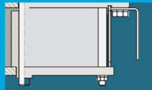
Desiccator to prevent ingress of moist air during vacuum operation
