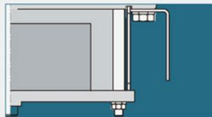
Floats on vacuum side preventing water ingress for installation of inerted ballast tanks
